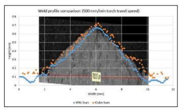
**Figure 4** Comparison of monitoring results with experimental macrographs.
