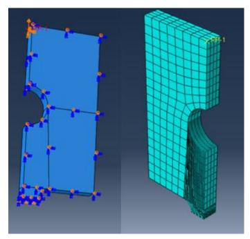
**Figure 2.** FEA boundary conditions and meshing size used to determine the effect of width of the waisted section, and loading hole diameter, on the elongation in the loading holes.
