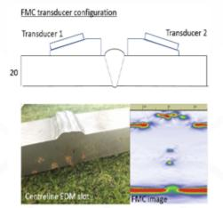
FMC girth weld setup, showing a 20mm thick plate weld containing a centreline electrical discharge machined (EDM) notch
