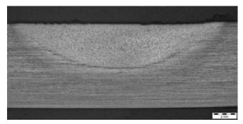
**Figure 2.** A macrograph of the BOP weld taken from the end of the wear assessment plate.
