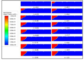
**Figure 1** Contour plot of liquid fraction at different times during the welding process.
