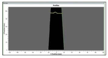
**Figure 3** Recorded weld bead dimensions as seen on screen using iCube Servo robot software.
