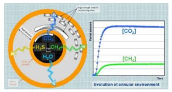
**Figure 1.** Evolution of annular environment through permeation.
