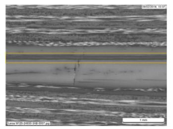
**Figure 1.** Sacrificial PEEK interlayer between two carbon/PEEK laminates. Yellow lines denote weld location.
