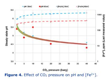
For a given test temperature and  $CO_2$  partial pressure, the pH increased with the concentration of dissolved iron concentration. The test solution remained supersaturated with iron throughout the duration of the experiments. The variation of [Fe2+] could be visualised in the aliquots removed (see Figure 5).
