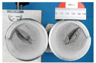
Figure 1. Fracture faces of a cracked M72 bolt.
