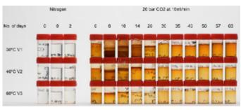
**Figure 5.** Visual indication of  $[Fe^{2+}]$  seen in aliquots extracted over the test duration.
