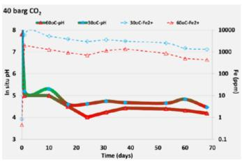
Figure 3. Solution pH and Fe concentration over time.
