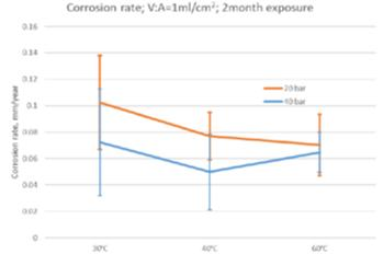
Figure 6. Corrosion rates calculated from mass loss.
