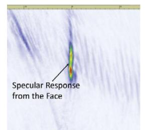
**Figure 2a** VSA image of a surface breaking flaw using Self-tandem using single mode. Here only the lower part of the flaw can be detected.
