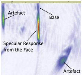
**Figure 2a** VSA image of a surface breaking flaw using the self-tandem multimode method. Here the base of the flaw can be distinguished.
