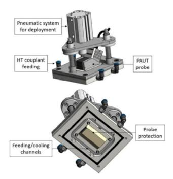
Figure 1. Prototype designed for EBW monitoring tool.
