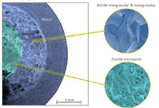
**Figure 1.** Fracture surface from a notched tensile specimen after slow strain rate testing (SSRT), tested under CP. A ring of brittle intergranular and transgranular fracture is shown around the circumference near the root of the notch.
