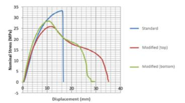
**Figure 3.** Examples of nominal stress vs displacement curves for the standard specimen geometry (EN 12814-7), and the modified specimen geometries for BF joints in 500mm SDR11 HDPE pipes (full thickness specimen cut in half to produce two specimens).
