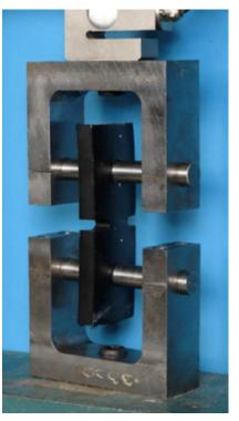
The energy to break the specimen is dependent on its wall thickness; as the thickness of the specimen increases, greater directional stresses (stress triaxiality) are generated, which decrease the ductility of the sample, even for the parent pipe. For this reason, the specimen geometry that is specified for joints in thin walled pipe will not be as discriminating for joints in thick walled pipe, because both good and poor quality joints will fail in a brittle or mixed manner.
