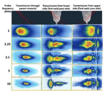
Figure 2. Results of the ultrasonic beam fingerprint.
