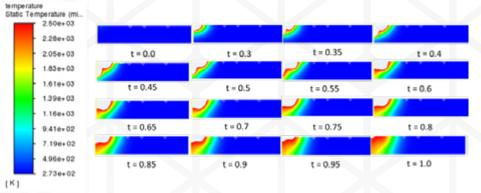
Contour plot of static temperature (K) at different times (s) during the welding process – travel speed: 500mm/ min
