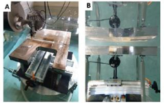
**Figure 1.** Ultrasonic beam fingerprint experimental setup on a welded component.
