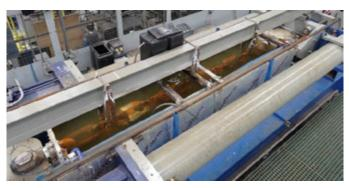
**Figure 1** Full-scale fatigue test set-up in free corrosion conditions in seawater.
